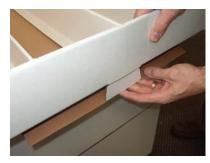
10) Place tray on base. Lock base flaps into slots on bottom of tray.
