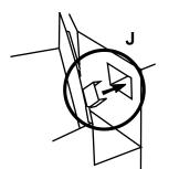
**5** Fold side flaps in toward each other as shown (I). Place bottom tray onto shelf and insert butterfly tabs into slots as shown (J). Repeat for second tier.
